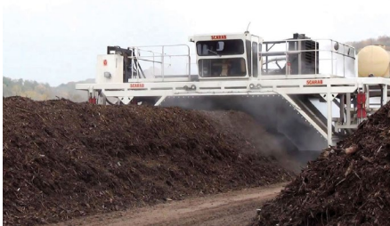
A Scarab works through a windrow of curing compost at the Solid Waste Agency compost facility.
